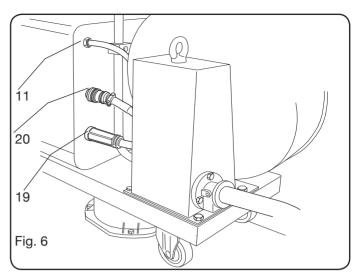
The coolant fluid hoses must be connected to the quick-fitting valves located below the lower part of the wire feeder trolley (see fig. 7), by matching the colours appearing on the trolley front side.
