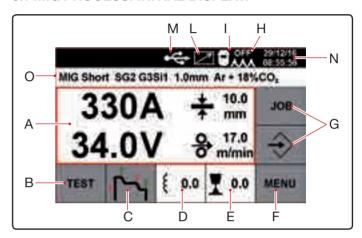
A The screen displays the welding current in Amperes, la welding voltage in Volts, the suggested thickness in mm and the welding wire speed in m/min. During welding the display shows the current and voltage values in a continuous manner and, once welding is completed, the last value in Amperes and Volts is displayed along with the HOLD word.
