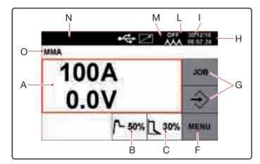
The screen displays the welding current in Amperes Aand the welding voltage in Volts.
