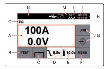
A The screen displays the welding current in Amperes and the welding voltage in Volts.
