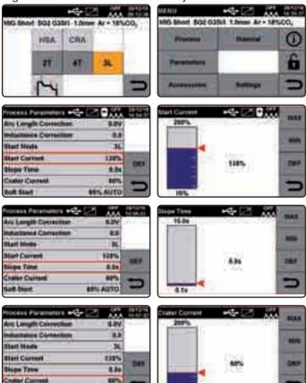
Press the key **DEF** to reset the factory set parameters.
