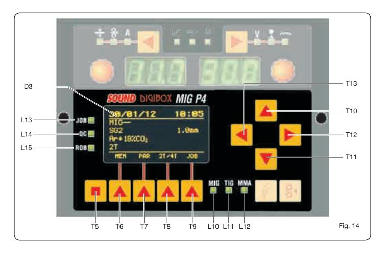
Immediately after it shows the values preset by the welding machine manufacturer:
