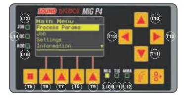
Programming is made in the "Main Menu". To access, press key **T5** and then key **T6 (MENU)** or through the quick access menu described under paragraph 8.
