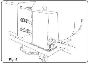
• The coolant fluid hoses must be connected to the quick-fitting valves located below the lower part of the wire feeder trolley (see fig. 7), by matching the colours appearing on the trolley front side.
