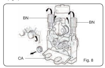
Open the door of the wire feeder compartment Remove the cover **CA** of the wire feeder unit.
