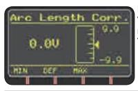
It allows to correct the Volt Arc length by means of keys **T10** and **T11** or knob**M2**.
